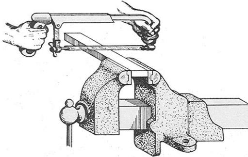
Fig. 16. Correct Position of Hands for Sawing with a Hand Hack Saw
